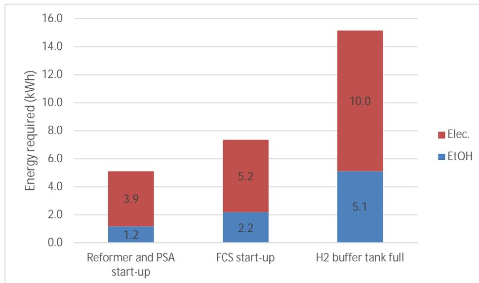
Figure 2: Electrical and thermal energy required for system start-up.
