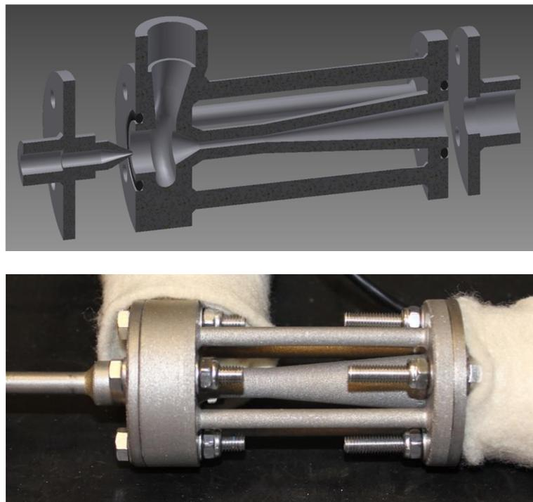
*Figure 4: Cross-sectional view of the custom ejector CAD model (top) and a photo of the manufactured ejector installed in experimental set-up (bottom).*
