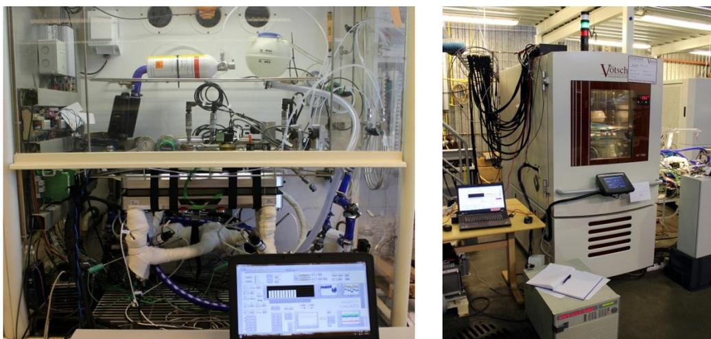
Figure 3: The S2 stack on impurity tolerance measurements (left) and under thermal stabilization preceding cold start-up (right).
